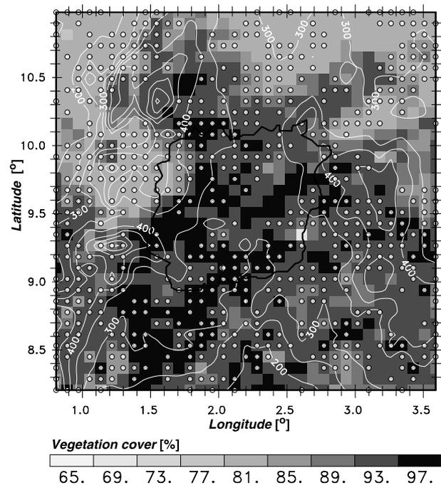
**Fig. 3.** Simulation domain with vegetation cover, orography (% , contour interval 50 m) and location of the HVO catchment. Grid points with altered SVAT quantities in the sensitivity runs are marked by white dots
