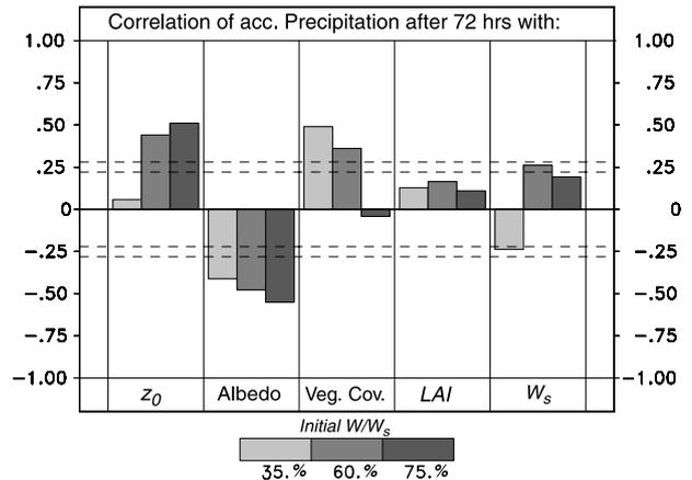
**Fig. 2.** Correlation of accumulated precipitation after 72 hours with SVAT parameters for sub-ensembles with equal initial soil water content. Dashed lines: 95% and 99% significance levels
