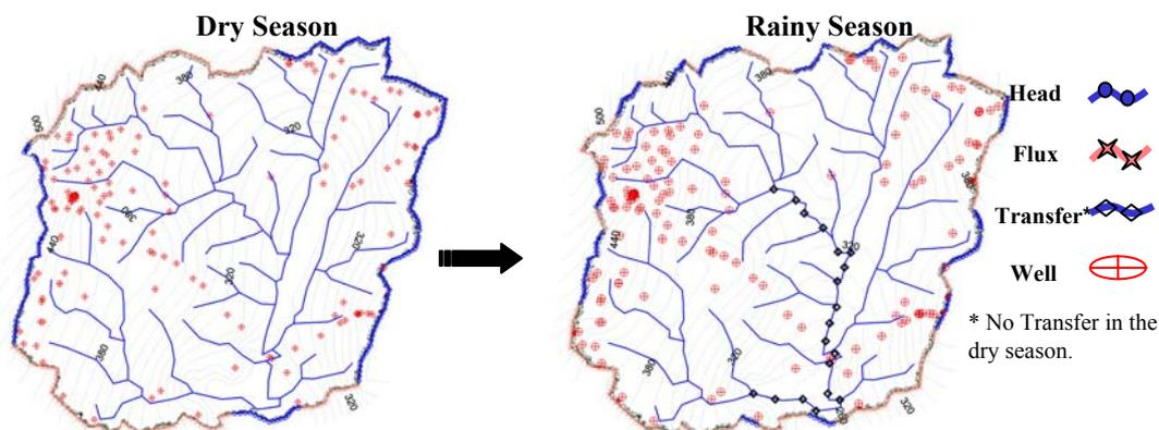
Fig. 5 Evaluation of the boundary conditions based on groundwater contour maps
