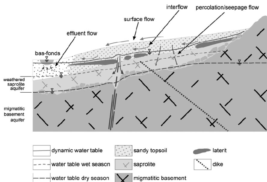
**Fig. 2** Hydrogeological conceptual model showing the major hydraulic processes.
