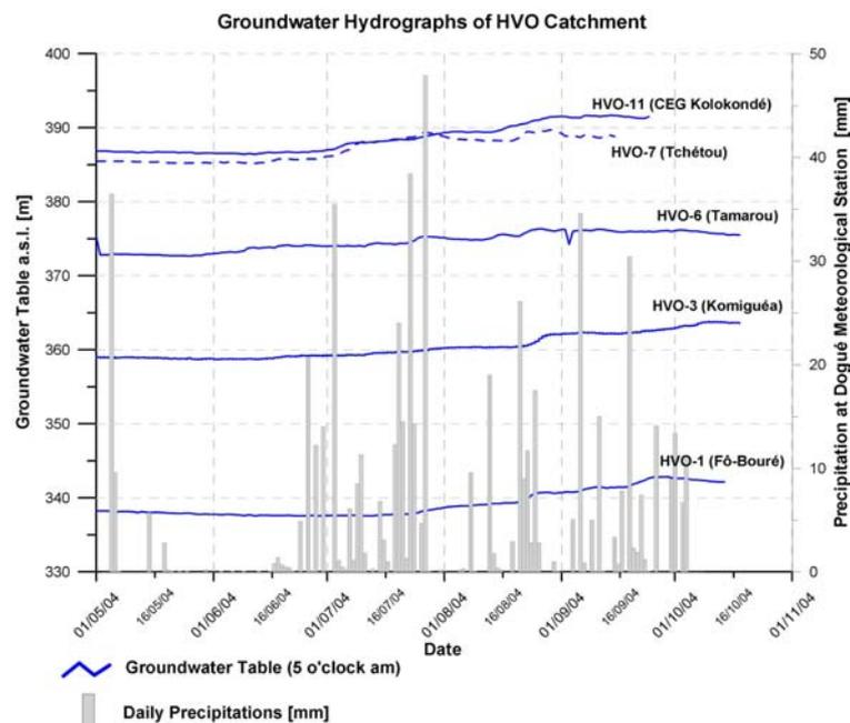
**Fig. 3** Hydrographs of some data logger in the Upper Ouémé catchment and rainfall measurements at Dogué showing the rain dependant rise of the water table.
